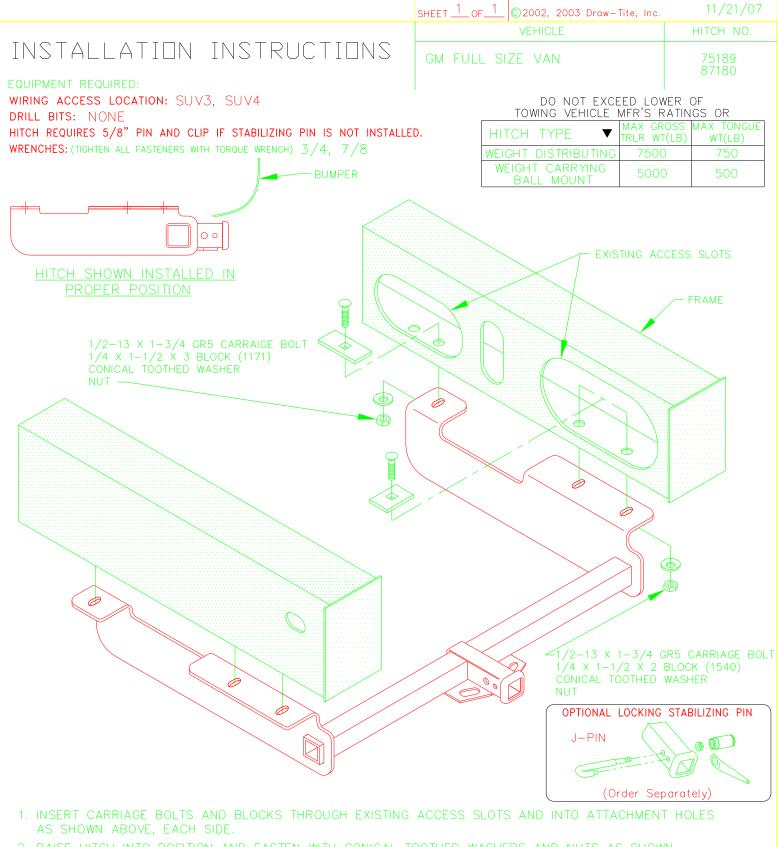
2. RAISE HITCH INTO POSITION AND FASTEN WITH CONICAL TOOTHED WASHERS AND NUTS AS SHOWN ABOVE, EACH SIDE.
