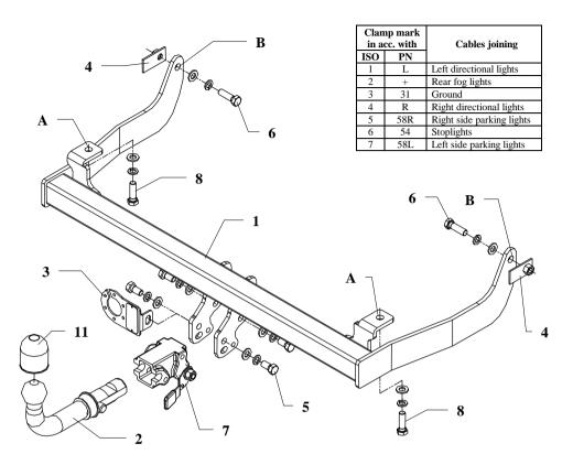
This towing hitch is designed to assembly in following cars: **VOLKSWAGEN CADDY II, SEAT INCA** both produced since 11.1995 till 12.2003, catalogue no. **K31A** and is prepared to tow trailers max total weight **1100kg** and max vertical load **50 kg**.
