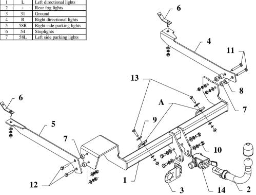
This towing hitch is designed to assembly in following cars: CITROEN XSARA ESTATE, produced since 1998 till 2005, catalogue no. P14A and is prepared to tow trailers max total weight 1300 kg and max vertical load 80 kg.
