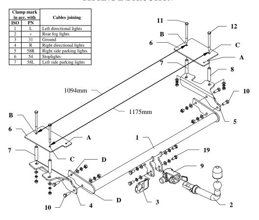
This towing hitch is designed to assembly in following cars: **FIAT PALIO WEEKEND ESTATE,** produced since 1998 till 2001, catalogue no. **R15A** and is prepared to tow trailers max total weight **1200 kg** and max vertical mass **70 kg**.
