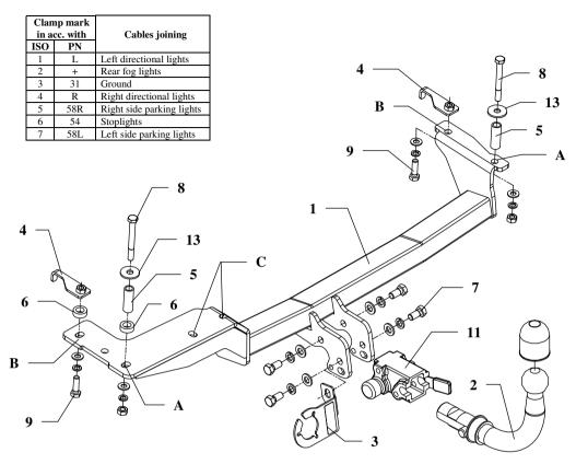
This towing hitch is designed to assembly in following cars: SEAT IBIZA 3/5 doors, produced since 04.1993 till 01.1996, catalogue number SC01A and is prepared to tow trailers max total weight 1100 kg and max vertical load 75 kg.
